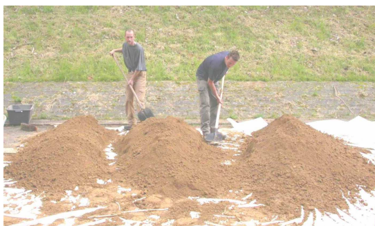
Figure 1: Quartering of the FSCC soil reference sample
