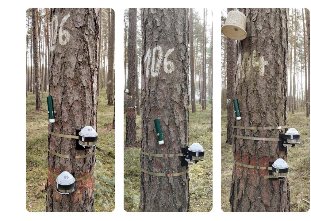
Fig 1 Girth band DB20 (above) and electronic band dendrometer DRL26 (below)
