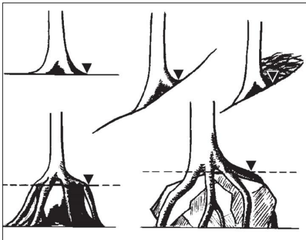
Figure 1: Definition of ground level under different conditions
