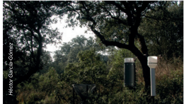
Figure 4-1: Collectors for wet deposition under the canopy (throughfall) of a holm oak forest near Madrid, Spain (Área Forestal de Tres Cantos, Ayto. Madrid).
